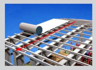
01. Unroll the insulation sheet, from bridge to eve (i.e. from the highest point to the lower).Stretch and fix the insulation sheet with drilling screws.
